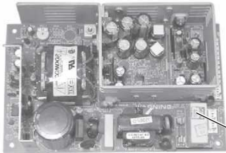
Power supply board
